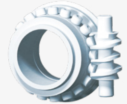
Swivel and indexing of the B-axis is driven by a servo motor and a roller gear cam, ensuring sufficient rigidity for powerful cutting as well as for high-precision positional control.
